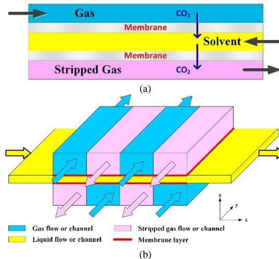
Fig. 1. HASMC configurations (a) Parallel-flow; (b) Cross-flow
