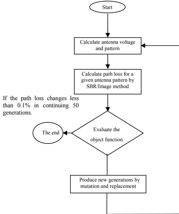
Fig.1. The flow chart for the simulation
