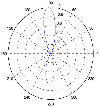
Fig. 3. Radiation pattern of Y array by the DDE algorithm (LOS case)
