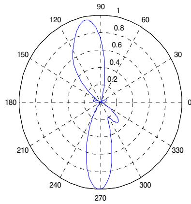
Fig. 4. Radiation pattern of L array by the DDE algorithm (NLOS case)
