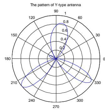
Figure 3(b). Radiation pattern by the DDE algorithm in the NLOS case
