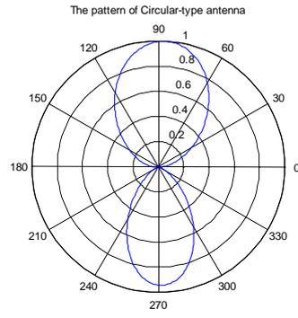
Figure 3(c). Radiation pattern by the DDE algorithm in the NLOS case
