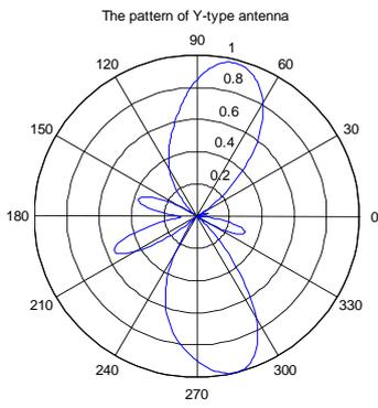
Figure 2(b). Radiation pattern by the GA algorithm in the NLOS case
