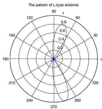
Figure 3(a). Radiation pattern by the DDE algorithm in the NLOS case
