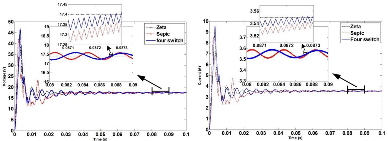
Figure 10. Voltage and current outputs from PV emulator for different buck-boost converter topologies loaded with 4.9  $\Omega$  resistor.
