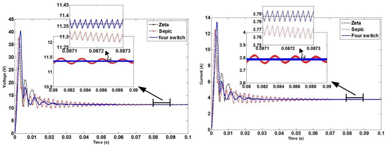
Figure 9. Voltage and current outputs from PV emulator for different buck-boost converter topologies loaded with 3  $\Omega$  resistor.
