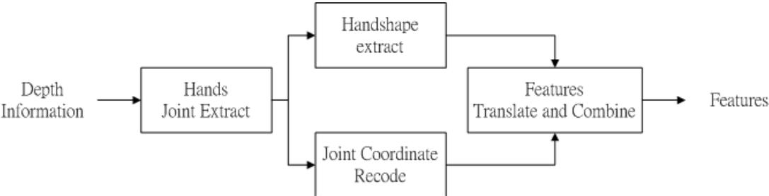
Fig.2: The detail flow chart of feature extraction
