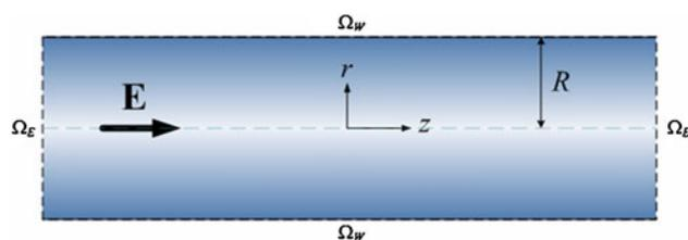
**Fig. 1** Electrokinetic flow along the axis of a cylindrical nanochannel of radius  $R$  subject to an applied uniform electrical field  $\mathbf{E}$  in the  $z$  direction;  $(r, z)$  are the computation domain of the cylindrical coordinates adopted with the origin on the axis of the channel;  $\Omega_W$  and  $\Omega_E$  are the channel wall and the input and output surfaces of that domain, respectively
