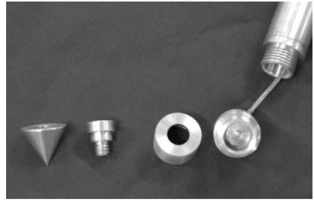
Figure 2 Decomposed elements of the load cell chamber
