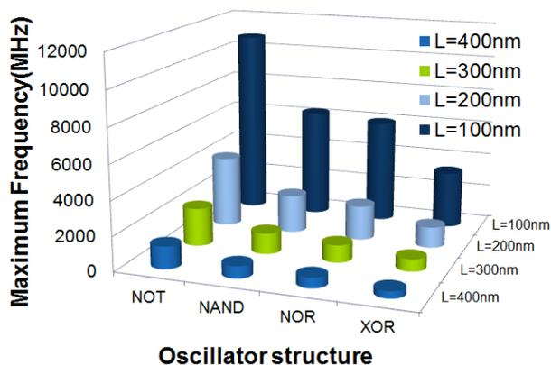
Fig. 11. Maximum frequency under FF, 1.0V, and -40°C.
