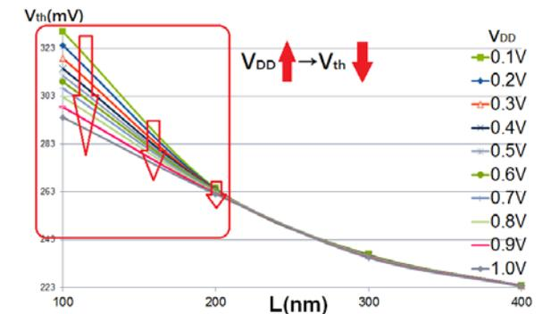
Fig. 5. The  $|V_{thp}|$  of PMOS of NOT gate.
