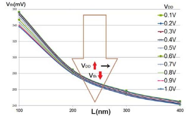
Fig. 4. The  $V_{thn}$  of NMOS of NOT gate.
