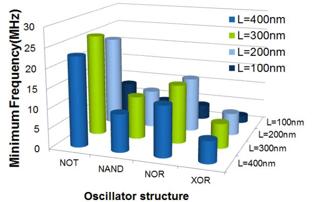
Fig. 10. Minimum frequency under SS, 0.3V, and -40°C.
