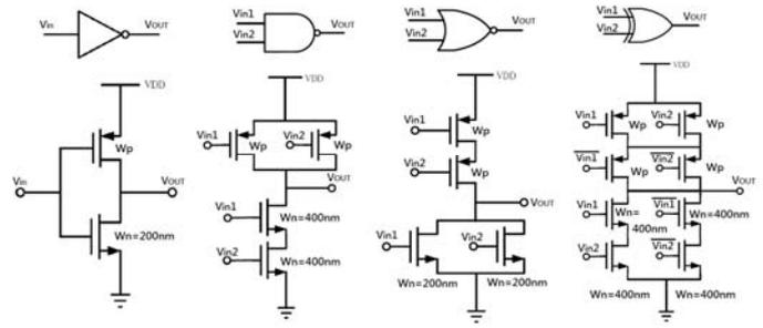
Fig. 2. Structures of NOT, NAND, NOR, XOR gates.
