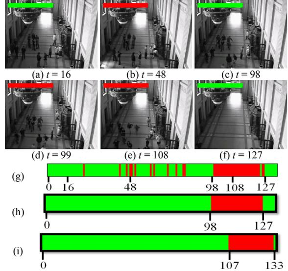
Fig. 3. Test result of test\_1; (a)-(f) are the frames of the detection results at time  $t$ , (g) is the complete detection result (without temporal smoothing), (h) is after temporal smoothing is applied, and (i) is the ground truth provided by UMN dataset and their normality transitions are about 1/3 second delay than ours..
