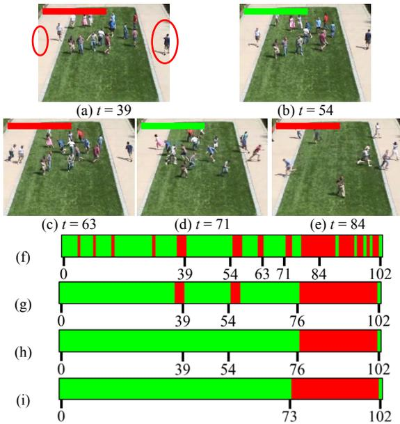
Fig. 4. Test result of test\_2; (a)-(e) are the frames of the detection results at time  $t$ , (f) is the complete detection result (without temporal smoothing), (g) & (h) are after temporal smoothing with  $r=2$  and  $r=3$ , respectively; (i) is the ground truth provided by UMN dataset.
