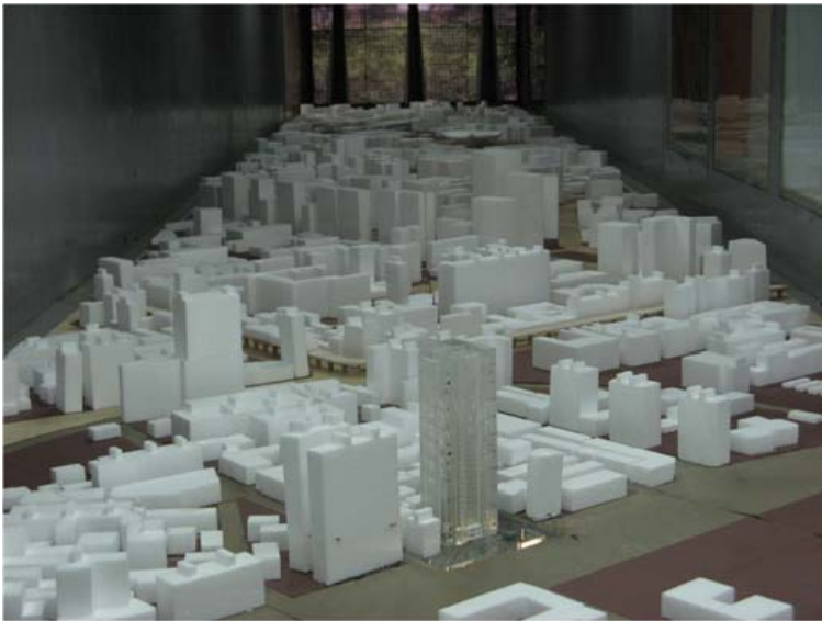
Figure 13: Wind tunnel model arrangement
