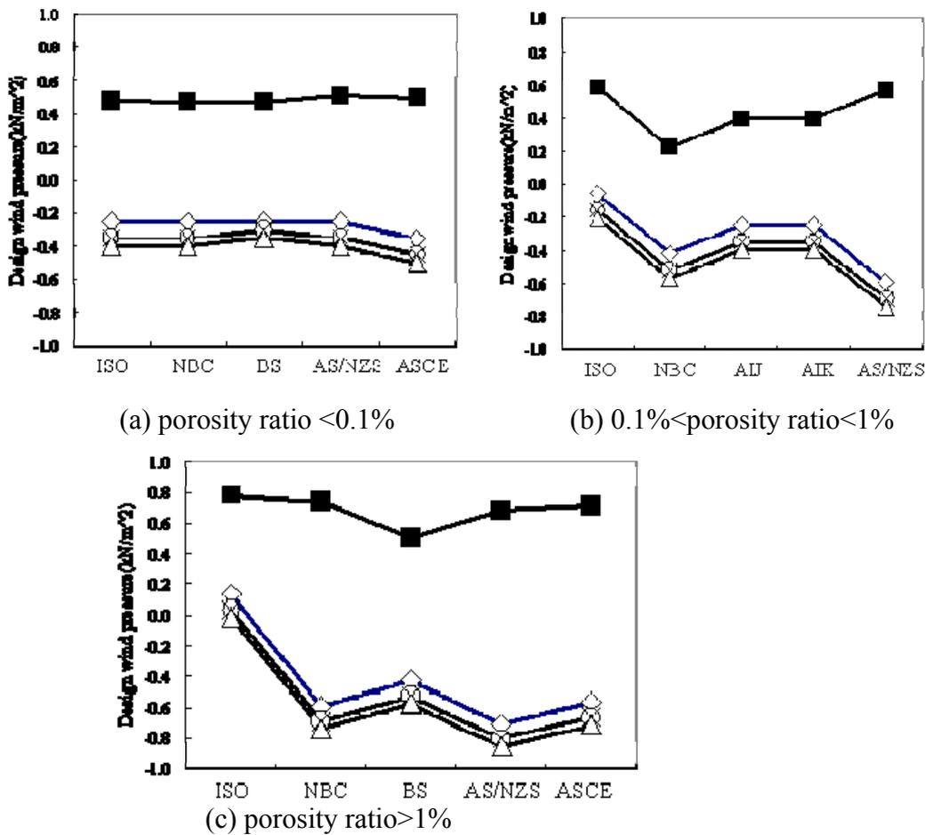
Figure 2 Design wind pressure for building with (a)small cracks, (b)small openings, (c)dominant opening. (■: windward wall, ◇: leeward wall, ○: side wall, △: windward roof, ×: leeward roof)
