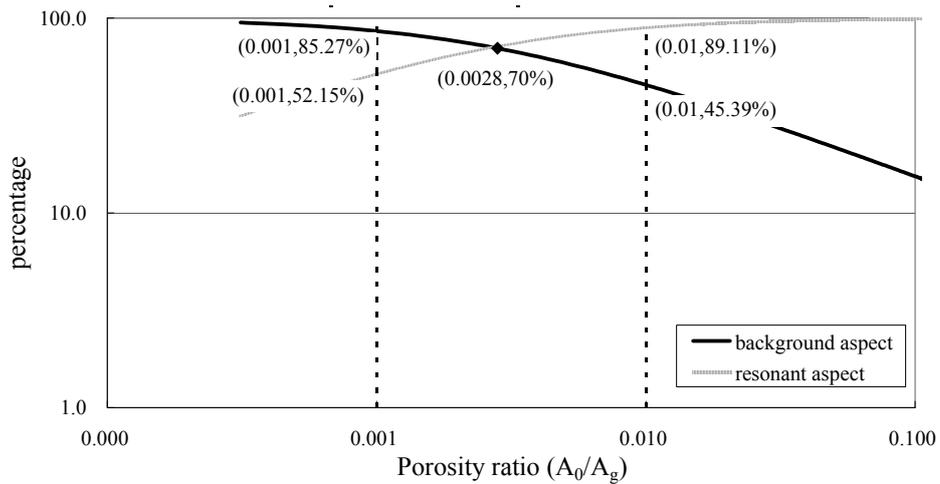
Figure 1 the percentage of background and resonant part of RMS internal pressure coefficient.
