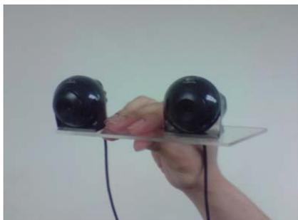
Figure 1. Binocular vision sensor system
