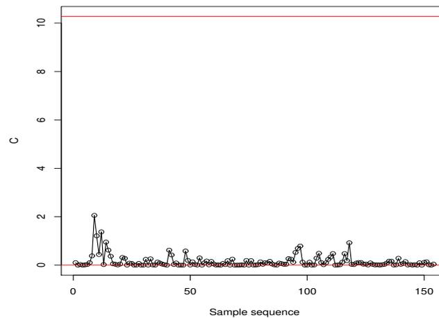
FIGURE 2. The BETA-chart for 153 vent-open profiles.
