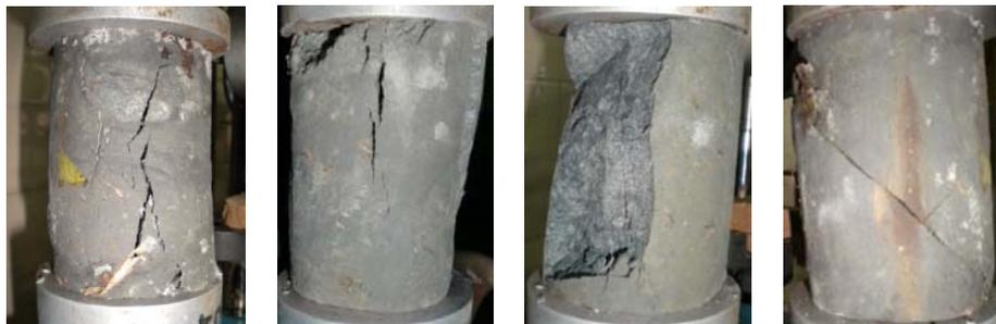
Figure 6. The typical stress-strain behavior of mudstone and fracture mode under compressive test.
