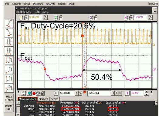
Fig. 8. Output waveforms of the proposed programmable frequency divider when  $F_{in}$  is 700MHz, the input divisor is 20, and the input duty-cycle is 20%.
