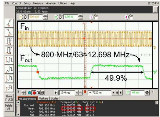
Fig. 7. Output waveforms of the proposed programmable frequency divider when  $F_{in}$  is 800MHz and the input divisor is 63.
