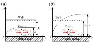
Fig.3 The illustration and notation of the dissolution tablets in the tube  $(a)\delta_c < R$ , $(b)\delta_c > R$ . Fig. 3 shows the conceptual diagram of the dissolved tablets in the CBL. A very small control volume was chosen to make a material balance on NaBH<sub>4</sub> (A) and the governing equation is shown below:
