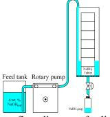
Fig. 1 Process flow diagram of solid sodium borohydride tablets dissolution systems.
