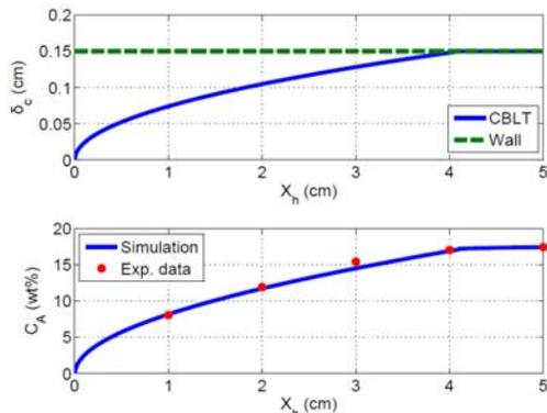
Fig. 4 (a) The concentration boundary layer thickness, (b) the average effluent  $\text{NaBH}_4$  concentration with respect to liquid level high.
