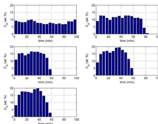
Fig. 2 The effluent  $\text{NaBH}_4$  concentration effect on liquid level of the tube (a)  $x_h = 1$  cm, (b)  $x_h = 2$  cm, (c)  $x_h = 3$  cm, (d)  $x_h = 4$  cm, (e)  $x_h = 5$  cm
