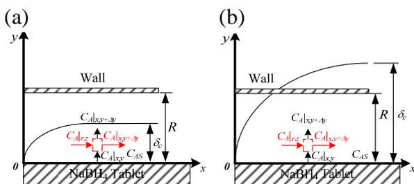
Fig.3 The illustration and notation of the dissolution tablets in the tube (a) $\delta_c < R$ , (b) $\delta_c > R$ .
