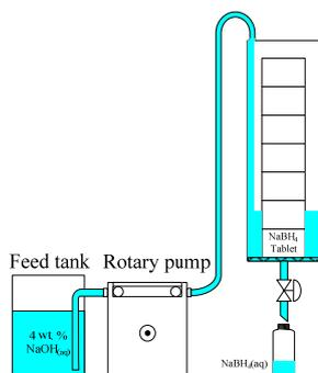
Fig. 1 Process flow diagram of solid sodium borohydride tablets dissolution systems.
