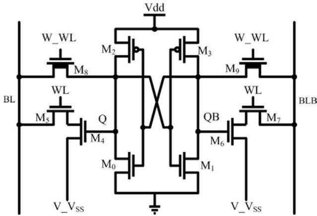
Figure 1. Proposed 10T SRAM cell.
