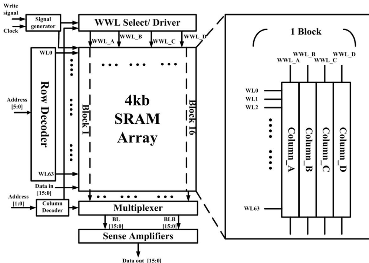
Figure 5. Architecture of the proposed SRAM and block structure of the proposed SRAM.
