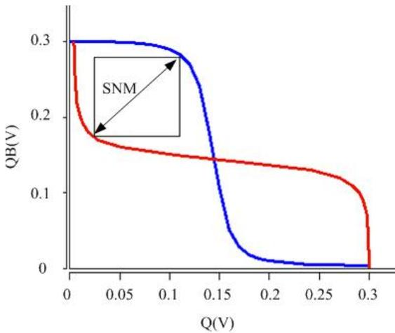
Figure 2. SNM of the proposed SRAM cell.
