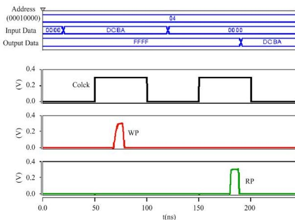
Figure 7. The simulation result of write data "DCBA" and read data "DCBA"
