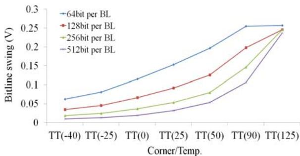
Figure 6. Analysis result of bit-line swing (with 300 mV power supply in typical process corner) at steady-state after WL enable
