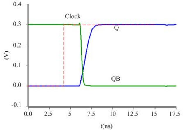
Figure 3. The simulation result of a single cell write operation.
