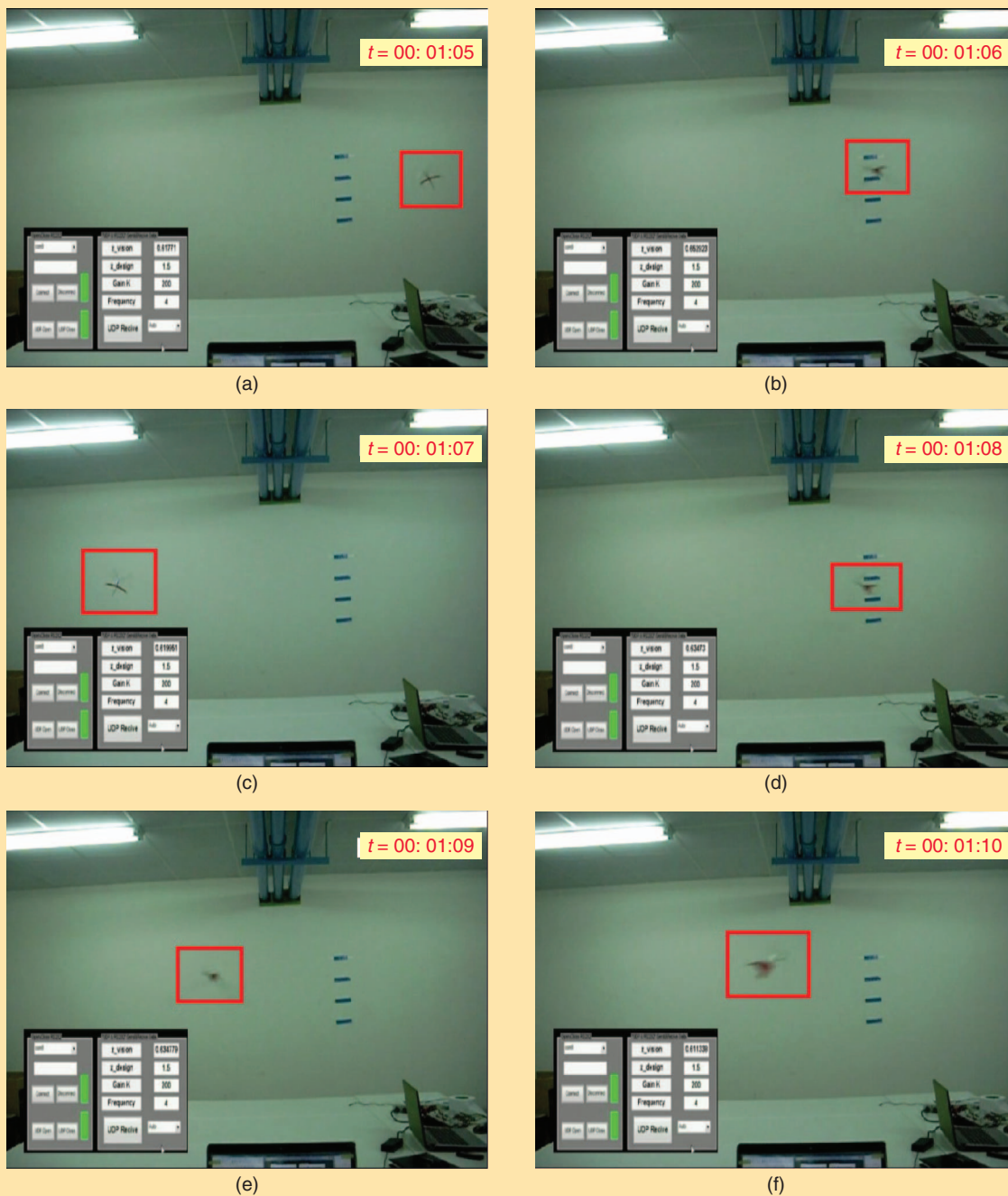
FIGURE 11 Flight tests in the laboratory. The micro aerial vehicle (MAV) is tethered to the ceiling with a string of negligible mass to force it to fly within a certain range. The blue stripes on the wall, denoting 1.8 m, 1.6 m, 1.4 m, and 1.2 m, respectively, from top to bottom, are set to provide visual references for human operators. The MAV is highlighted by a red circle. The MAV flies around the preassigned cruise altitude h = 1.5 m. These pictures are snapshots from a video [24]. The MAV is highlighted and the clock was post-edited with a photo editor.
