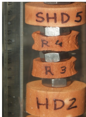
Fig. 1. Pressure test for Foam compressibility
