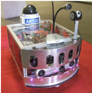
Fig. 1. A utonomous R obot for T ransport and S ervice, equipped with laser scanner and ultrasonic sensors
