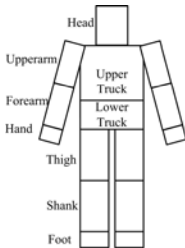
Fig. 1. Hanavan's human body model Fig. 2. Coordinate system definition of human leg
