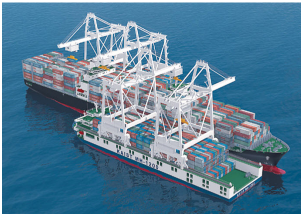
Fig. 1. Mobile harbor can load/unload containers at sea using its crane
