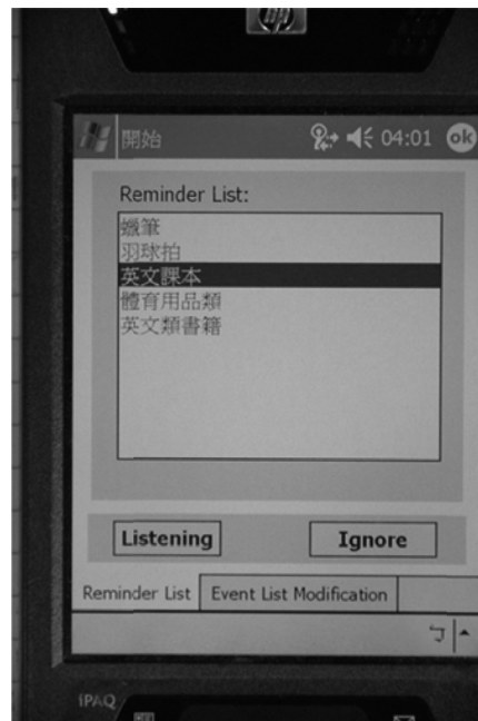
Fig. 5. The reminder list sent by the server is displayed on the client PDA.
