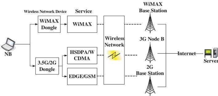
**Figure 5.** Functional block diagram for system performance simulation.
