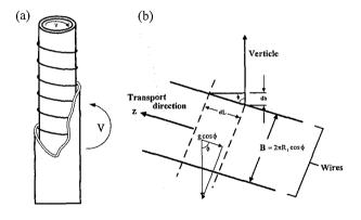
Fig. 2. Spiral wire inserted as a spacer in the annulus of a concentric-tube thermal-diffusion column. (a) Wired column with tubes rotated; (b) transport direction.
