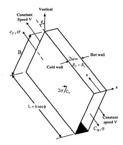
Fig. 3. Moving-wall parallel-plate column inclined on edge.
