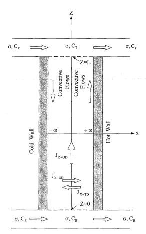
Fig. 1. Transverse-flow flat-plate thermal-diffusion column.
