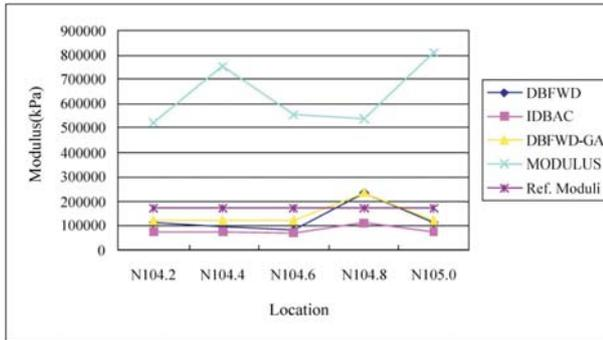
**Figure 6.** Comparative subbase layer backcalculation results for FWD measurements on case study.
