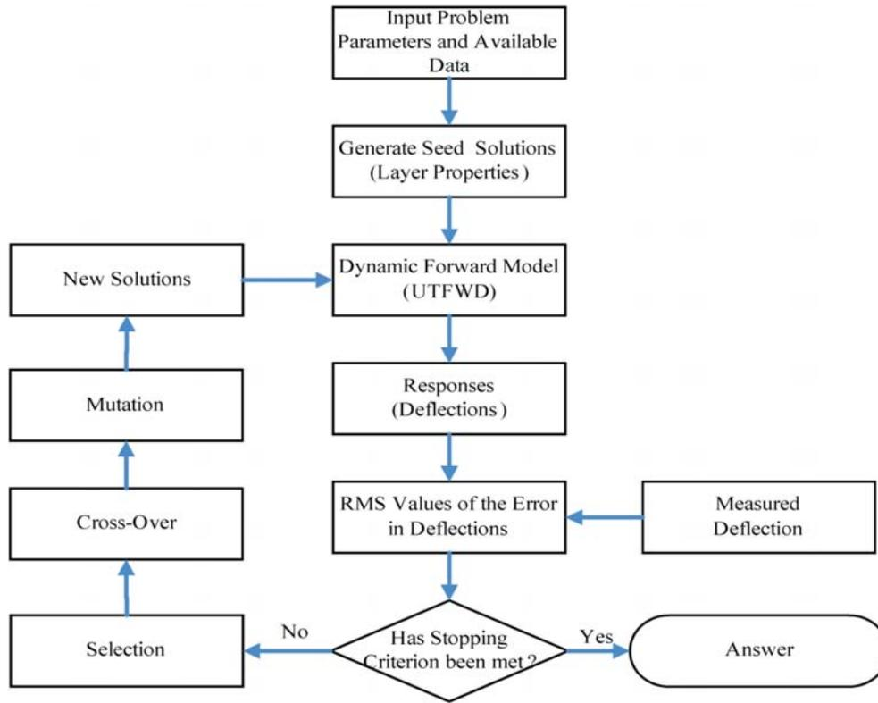
Figure 2. Flowchart of genetic algorithm based on backcalculation program DBFWD-GA.
