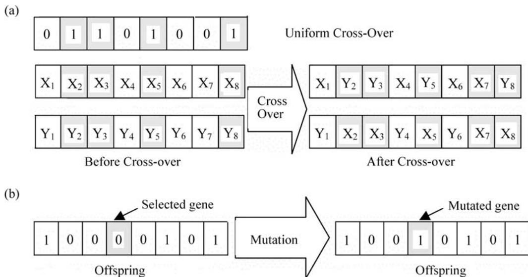
Figure 1. Examples of GA operations: (a) Uniform Cross-Over; (b) mutation.
