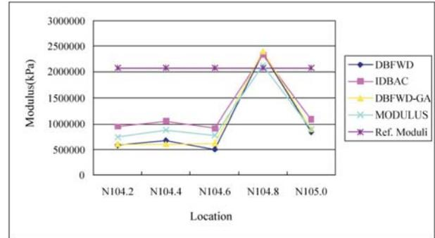
**Figure 5.** Comparative base layer backcalculation results for FWD measurements on case study.
