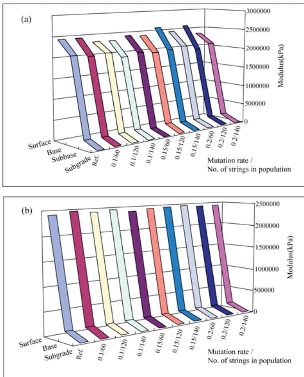
**Figure 3.** Comparative backcalculation results for pavement structure considering various mutation rate and population number: (a) 4-layer; (b) 3-layer.
