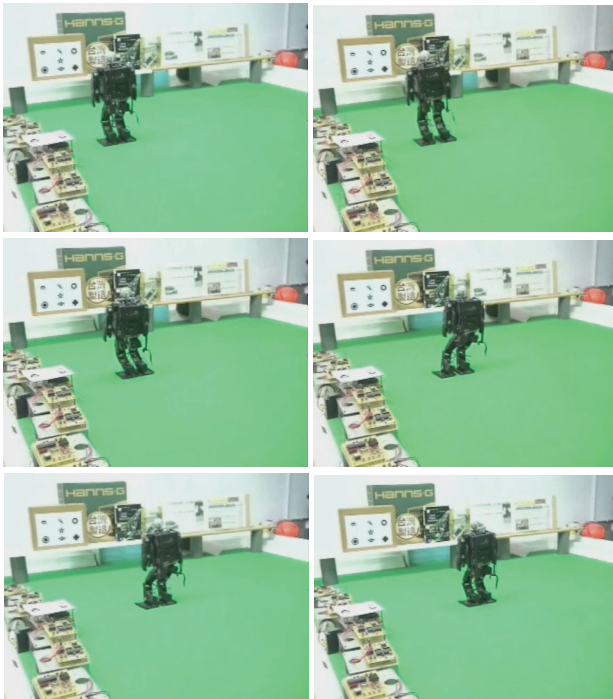
Fig. 7. Humanoid robot moves from left- to right-side of the field. Meanwhile, the EKF-based visual SLAM is performed
