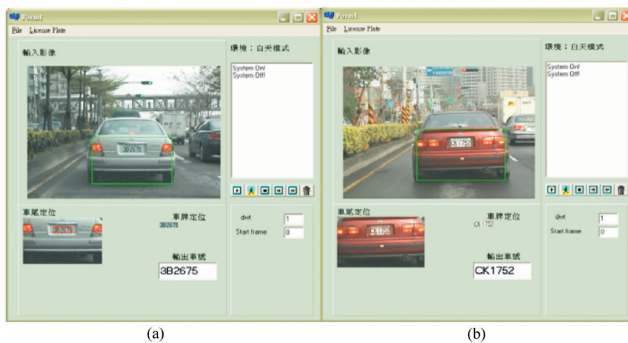
Figure 11. (a) The recognition result for complicated background, (b) The recognition result for red and tilted vehicle body.
