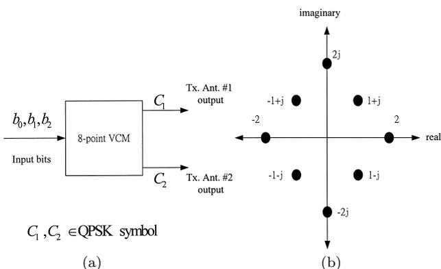
**Fig. 3** (a) The virtual constellation mapping function block and (b) is the 8-point signal constellation.
