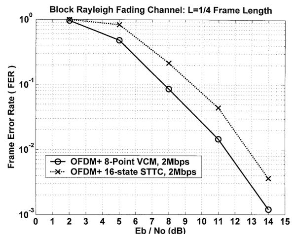
**Fig. 8** FER performance comparison of the 8-point VCM OFDM scheme and the space-time coded OFDM scheme in the block Rayleigh fading channel.
