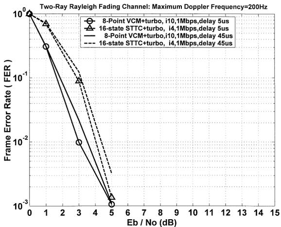
Fig. 10 FER performance comparison of the STTC concatenated turbo code OFDM scheme and the 8-point VCM OFDM scheme in the two-ray fading channels.
