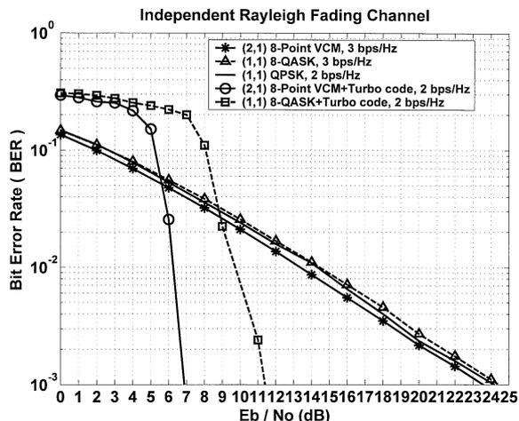
**Fig. 5** The BER performances of the 5 different transmit schemes in Rayleigh fading channel. The turbo coded frame length is 512 bits, and decoding iteration number is 4.
