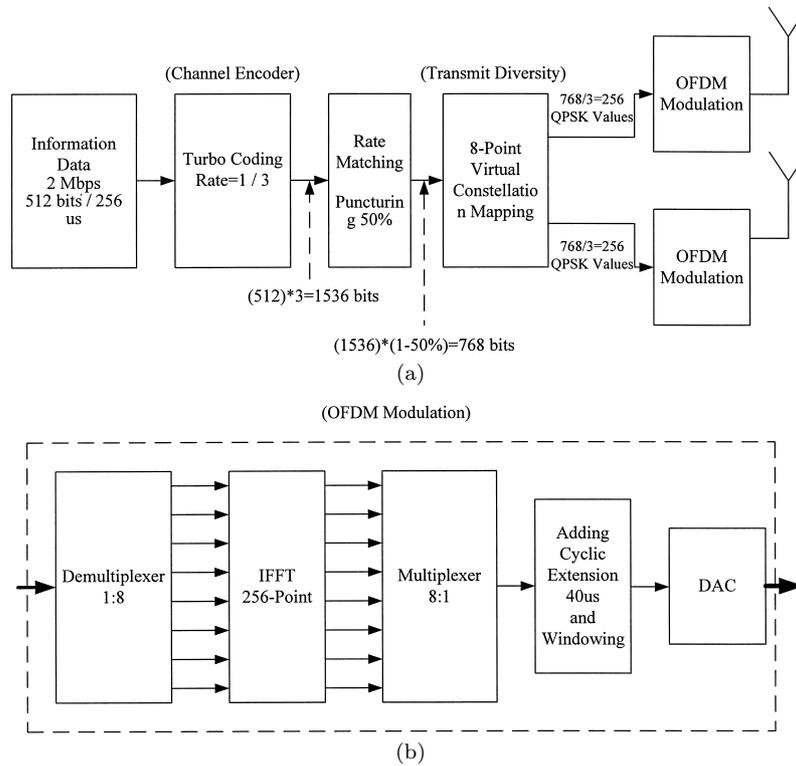
Fig. 6 (a) The OFDM downlink 2 Mbps framework is formed with the turbo code and the 8-point VCM and (b) is the OFDM modulation structure.
