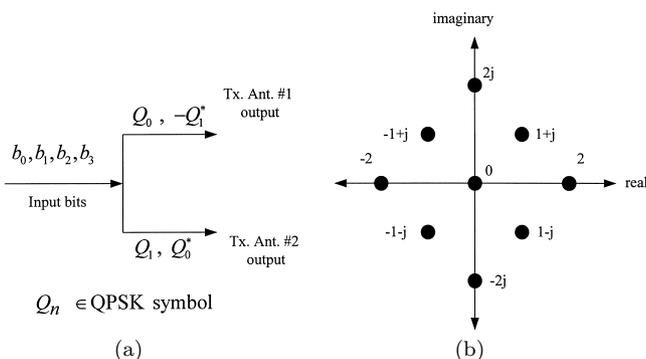
**Fig. 2** (a) The STBC encoder block diagram and (b) is a 9-point signal constellation, that is air combined two transmitted QPSK symbols from Ant. #1 and Ant. #2 in one QPSK symbol period.
