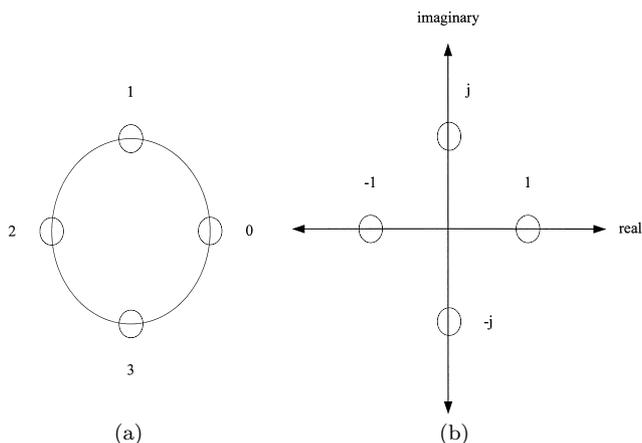
**Fig. 1** (a) The QPSK signal constellation and (b) is its real and imaginary part.
