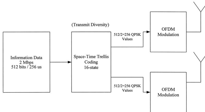
Fig. 7 The OFDM downlink 2 Mbps framework employs a 16-state space-time trellis code [8].
