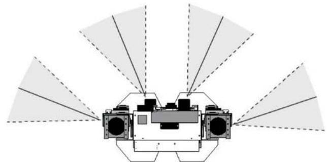
**Figure 10.** Detectable ranges of four infrared sensors.
