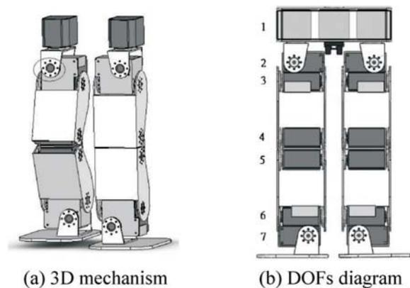
Figure 7. Legs mechanism of TWNHR-III.
