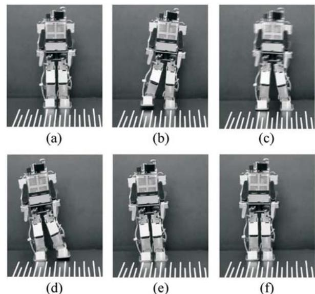
Figure 14. Slipping to the right side of TWNHR-III.
