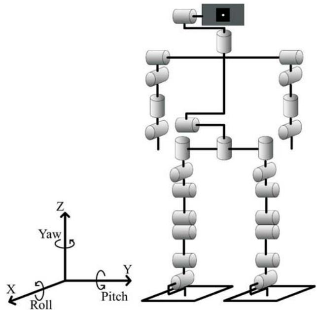
Figure 1. DOF configuration of TWNHR-III.
