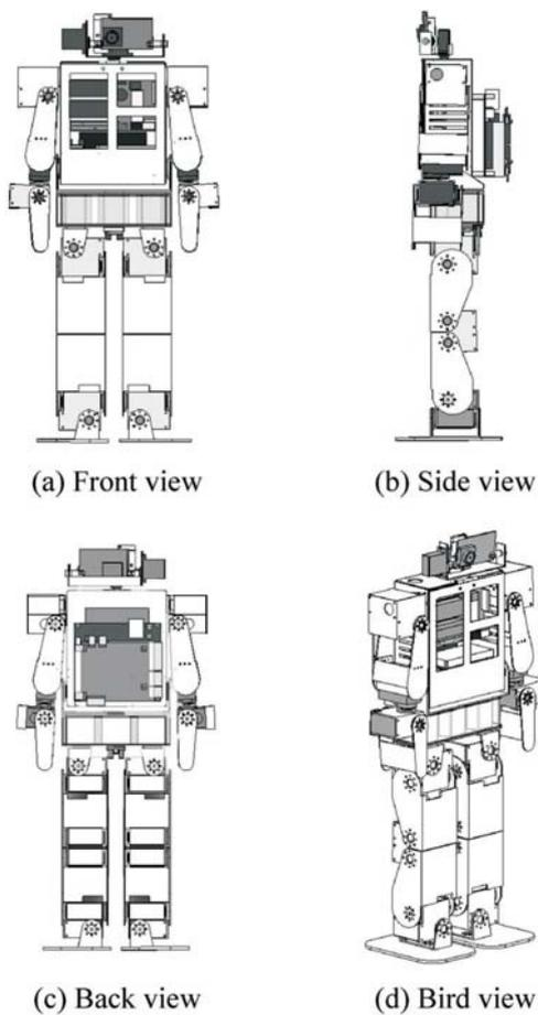
**Figure 3.** Views of TWNHR-III from 3D mechanism design.
