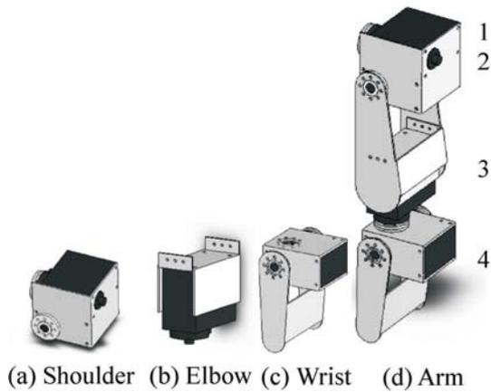
Figure 6. Left arm mechanism of TWNHR-III.
