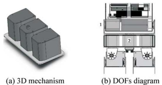
**Figure 5.** Waist and trunk mechanism of TWNHR-III.
