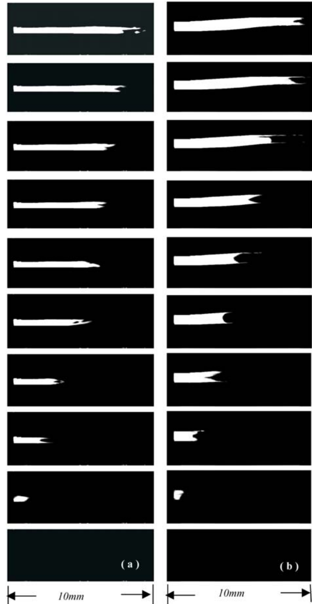
Figure 7. Plot (a) and (b) to show the continuous pictures of healed line- and cross-crack during mass transfer at 50 °C.
