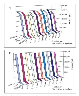
Figure 3. Comparative backcalcualtion results for pavement structure considering various mutation rate and population number: (a) 4-layer; (b) 3-layer.
