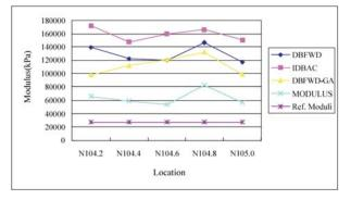
Figure 7. Comparative subgrade layer backcalculation results for FWD measurements on case study.
