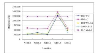
Figure 4. Comparative surface layer backcalculation results for FWD measurements on case study.
