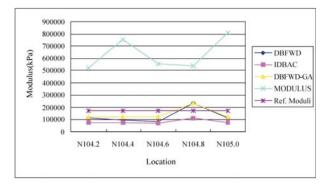
Figure 6. Comparative subbase layer backcalculation results for FWD measurements on case study.
