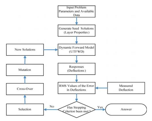
Figure 2. Flowchart of genetic algorithm based on backcalculation program DBFWD-GA.
