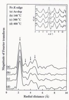
data at the Fe K-edge from k=3.2 to 11  ${\rm \AA}^{-1}$  for the asdeposited and three annealed NiFe-FeMn bilayers. The inset represents the Fe  $K\text{-}\mathrm{edge}$  EXAFS oscillation  $k^3\chi$ data.
