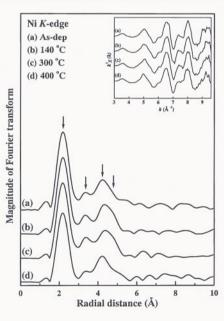
data at the Ni K-edge from k=3.2 to  $9.7~{\rm \AA}^{-1}$  for the asdeposited and three annealed NiFe-FeMn bilayers. The inset represents the Ni K-edge EXAFS oscillation  $k^3\chi$
