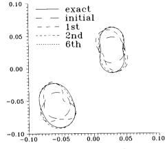
Fig. 6. Shape functions for example 2. The solid curve represents the exact shape, while the dashed curves are calculated shapes in iteration process.
