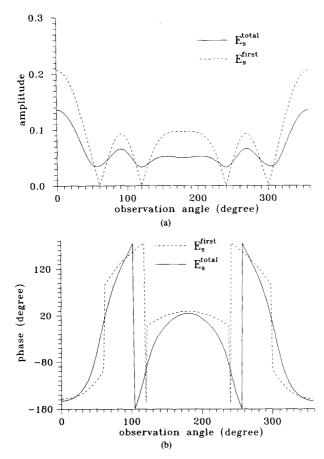
Fig. 2. First-order and total scattered fields for the incident angle  $\phi = 90^{\circ}$ . (a) Amplitude. (b) Phase.
