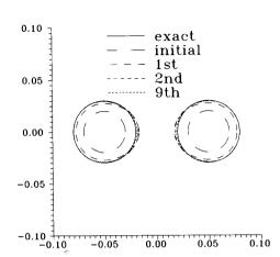
Fig. 3. Shape functions for example 1 with  $d_1 = d_2 = 0.05$  m. The solid curve represents the exact shape, while the dashed curves are calculated shapes in iteration process.
