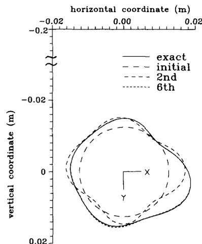
Fig. 2. Shape functions for object  $A$  buried in the soil ( $\epsilon_2 = 2.55\epsilon_0$  and  $\sigma_2 = 2 \times 10^{-2}$  S/m) at a depth of  $a = 2\lambda_0$ . The solid curve represents the exact profile, while the dashed curves are calculated profiles in the iteration process.
