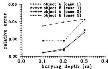
Fig. 4. Reconstruction error as a function of burying depth with two different soil parameters; case 1: ( $\epsilon_2 = 2.55\epsilon_0$  and  $\sigma_2 = 2 \times 10^{-3}$  S/m), case 2: ( $\epsilon_2 = 2.55\epsilon_0$  and  $\sigma_2 = 2 \times 10^{-2}$  S/m).
