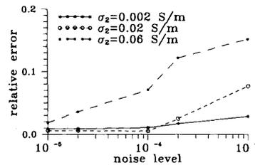
Fig. 6. Reconstruction error as a function of noise level at a burying depth of  $a = 2\lambda_0$  for object *A* in three different soils.
