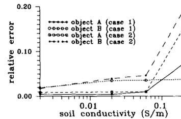
Fig. 5. Reconstruction error as a function of soil conductivity at two different burying depths; case 1:  $a = \lambda_0$ , case 2:  $a = 2\lambda_0$ .
