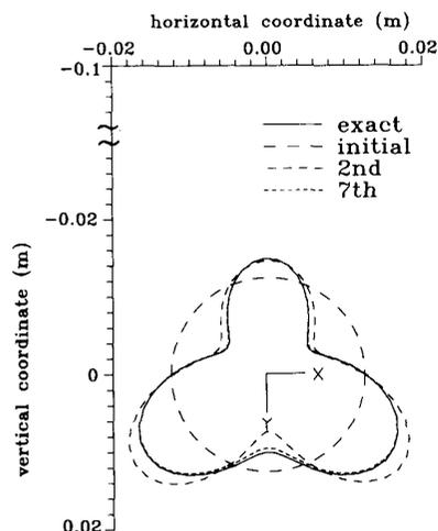
Fig. 3. Shape functions for object  $B$  buried in the sandy soil ( $\epsilon_2 = 2.55\epsilon_0$  and  $\sigma_2 = 2 \times 10^{-3}$  S/m) at a depth of  $a = \lambda_0$ . The solid curve represents the exact profile, while the dashed curves are calculated profiles in the iteration process.
