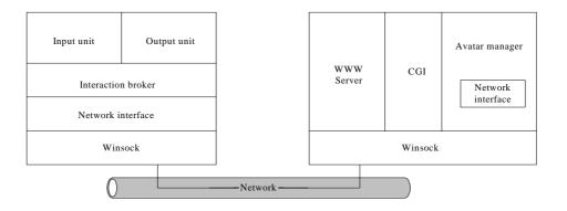
Figure 2. The infrastructure of a web-based multi-user system
