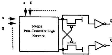
Fig. 5. Basic CPL circuit schematic structure
