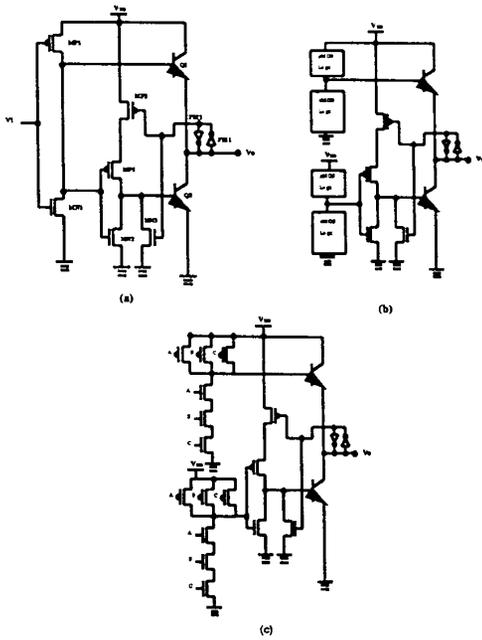
Fig. 2. Feedback-controlled enhance-pull-down BICMOS (FC-EPD-BICMOS) (a) inverter; (b) general structure; (c) 3-input NAND gate.
