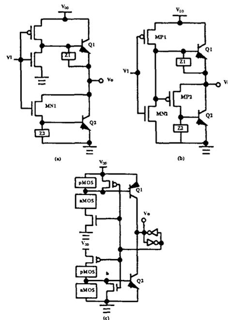
Fig. 1. Schematic circuits of (a) conventional (Darlington-type) BiCMOS inverter (b) QC-BiCMOS inverter (c) TS-BiCMOS
