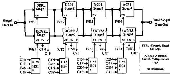
Figure 7. Structure of the Micro-Pipeline with the New Handshake Methodology.
