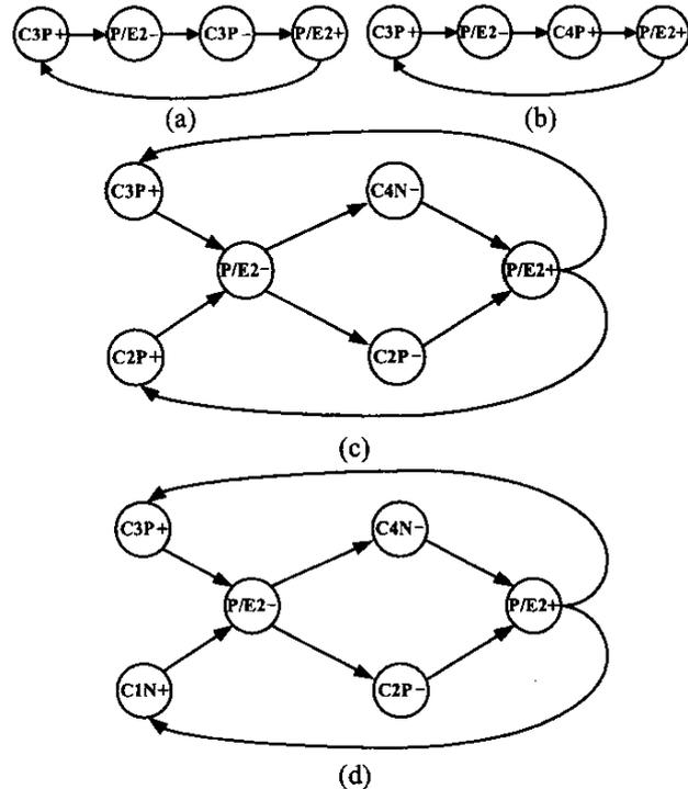
Figure 3. Handshake Signal Transition Graphs. (a) Williams. (b) Matsubara, Ide and Singh, Nowick's LP3/1. (c) Chan. (d) The Proposed Handshake.
