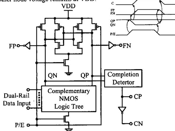
Figure 1. DCVSL Circuit with Completion Detector, Dynamic Sense Amplifier, and Timing Diagram.
