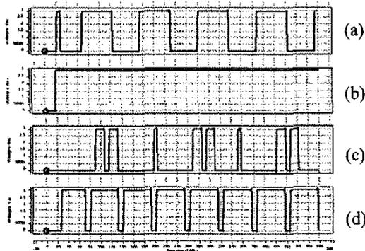
Figure 8. Simulation results of P1. (a) Williams. (b) Matsubara, Ide and Singh, Nowick's LP3/1. (c) Chan. (d) The Proposed Handshake.
