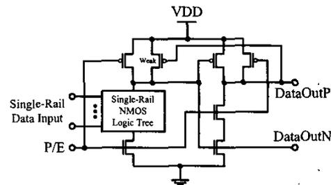
Figure 5. Dynamic Single-Rail Logic (DSRL) Circuit.
