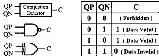
Figure 2. Completion Detector Circuit and Truth Table.
