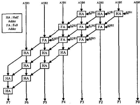
Figure 6. Architecture of Micro-Pipeline Multiplier.
