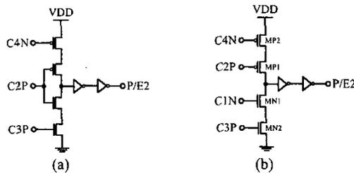
Figure 4. Handshake Circuits. (a) Chan. (b) The Proposed Handshake.
