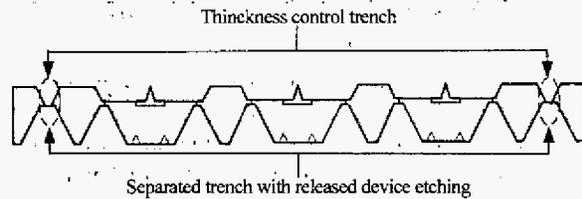
Figure 5: The cantilever thickness control of  $3 \times 5$  AFM probes array by liquid-based gravity-driven etching-stop technique.
