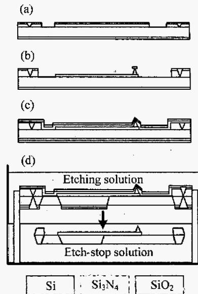
Figure 6: The detailed fabrication and thickness control process of the silicon-based AFM probes array: (a) the cantilever beam and thickness control trenches fabrications; (b) the squares silicon nitride act as a mask against an anisotropic etchant of KOH; (c) The apex of the pyramids are sharpened by re-oxidation and protection layer deposition; (d) the probes array chip released with the gravity-driven thickness-controlled technique.
