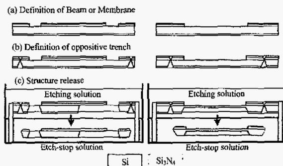
Figure 2: The fabrication and thickness control processes of microstructure: (a) the definition of microstructure; (b) the manufacture of opposite trenches for the thickness control; (c) the device release with thickness control technique.
