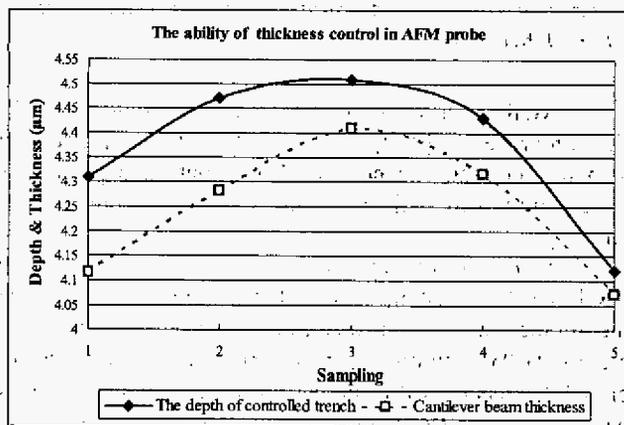
Figure 8: The dimension deviation of the proposed thickness of cantilever beam with respect to the depth of controlled trench.
