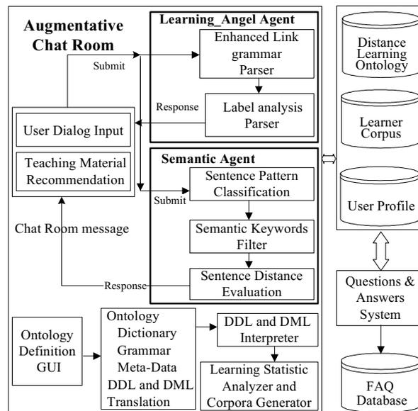
Fig. 3 The system architecture and operation flow
