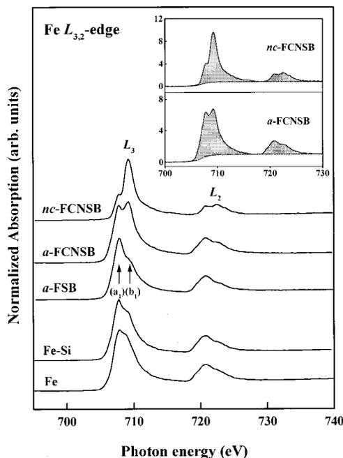
FIG. 2. Normalized Fe  $L_{3,2}$  near-edge absorption spectra of *nc*-FCNSB, *a*-FCNSB, *a*-FSB, and Fe-Si. The integrated area of shaded regions represents the extrapolated background at the Fe  $L_3$  edge for *nc*-FCNSB and *a*-FCNSB, as shown in the inset. These areas are used to calculate the  $I(L_3)$  and  $I(L_2)$ . The center of the continuous step of the arctangent function was selected at the inflection point of the threshold.
