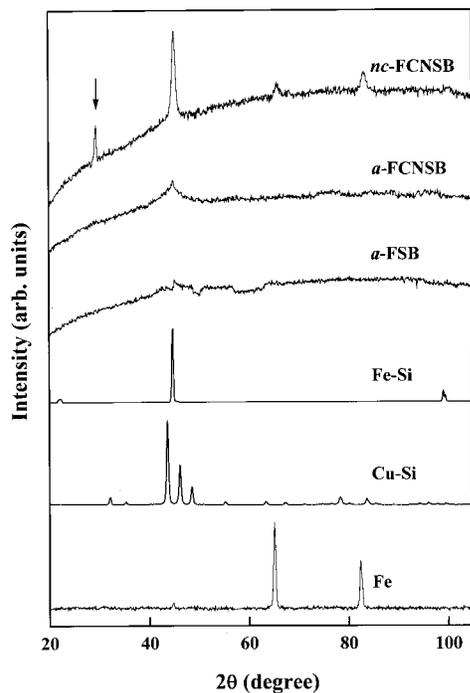
FIG. 1. Representative x-ray-diffraction spectra of *nc*-FCNSB, *a*-FCNSB, *a*-FSB, Fe-Si, Cu-Si, and Fe metal.
