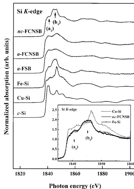
FIG. 5. Normalized Si  $K$  near-edge absorption spectra of  $nc$ -FCNSB,  $a$ -FCNSB,  $a$ -FSB, Fe–Si, Cu–Si, and  $c$ -Si (the data for  $c$ -Si were measured using the sample drain current mode). The inset shows a comparison of the Si  $K$ -edge XANES spectrum of  $nc$ -FCNSB, Fe–Si, and Cu–Si.
