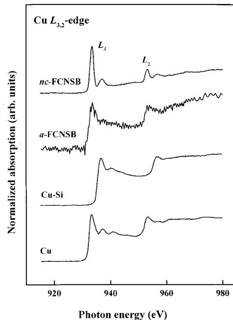
FIG. 3. Normalized Cu  $L_{3,2}$  near-edge absorption spectra of *nc*-FCNSB, *a*-FCNSB, Cu-Si, and Cu metal (the data for Cu metal were measured using the sample drain current mode).
