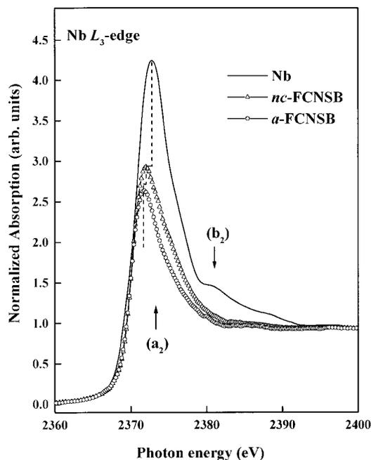
FIG. 4. Normalized Nb  $L_3$  near-edge absorption spectra of  $nc$ -FCNSB,  $a$ -FCNSB, and Nb metal (the data for Nb metal were measured using the sample drain current mode).
