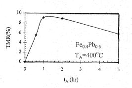
Fig. 3 Magnetoresistance effect(TMR) versus  $t_A$  for Fe-Pb-O granular films. The measurement temperature is 300K. The applied field is 0.9Tesla.
