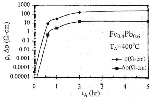
Fig. 2 Resistivity  $\rho$  at 300K and the absolute value of  $\Delta\rho$  versus  $t_A$  for Fe-Pb-O granular films. The vertical axis is plotted in a logarithmic scale. The applied field is 0.9Tesla.
