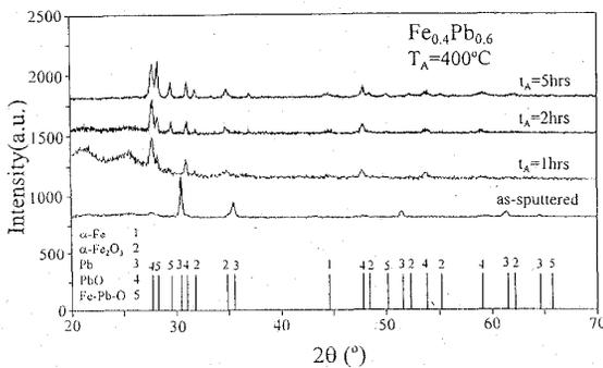
Fig. 1 Representative X-ray diffraction patterns for the Fe-Pb-O granular films. The films are annealed at 400°C with different annealing time.
