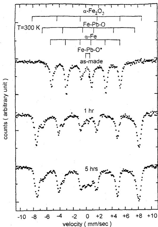
Fig. 4 Mössbauer spectra for the Fe-Pb-O granular films at 300K.
