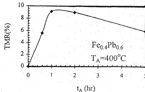
Fig. 3 Magnetoresistance effect(TMR) versus  $t_A$  for Fe-Pb-O granular films. The measurement temperature is 300K. The applied field is 0.9Tesla.
