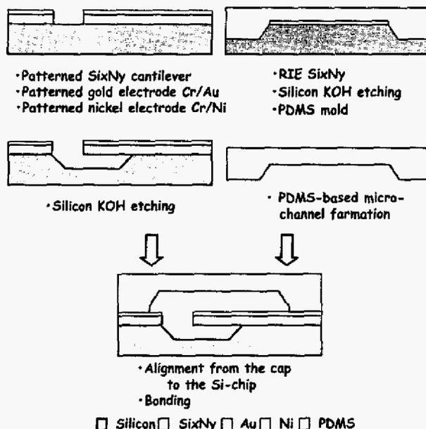
Figure 2: Fabrication process flow of micro-cantilever bio-detection chips.
