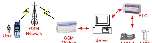
Fig. 1 The system overview of the designed M-PLC control lab using GSM system
