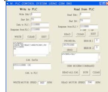
Fig. 2 Control and monitor interface in server end
