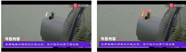
Fig. 12 Maximum delay of 0.5 second after the fire starts (Left image shows the beginning of the fire, right image shows the detection after 0.5 second)
