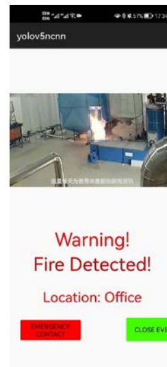
Fig. 15 Warning displayed when a fire is detected
