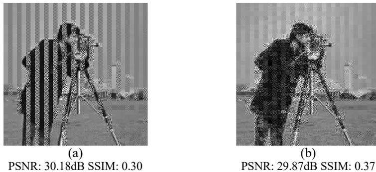
**Fig. 5.** Simulations of reconstructed image qualities for BCS with adaptive sampling under the  $L_2$  constraint for lossy rate of 50%. (a) No protection applied. (b) Protection with MDTC.
