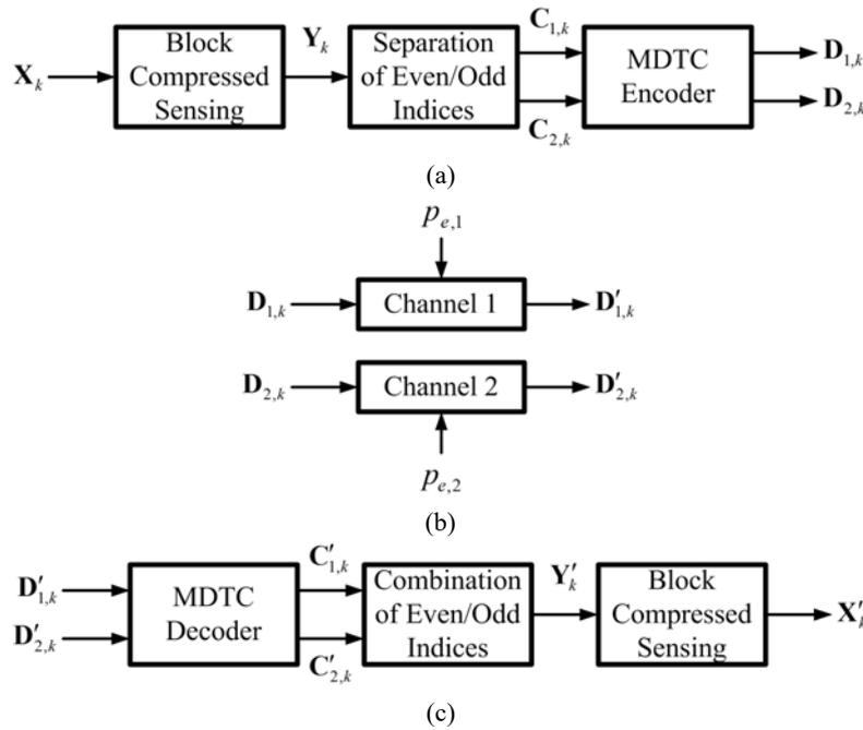
Fig. 1. Block diagrams for transmission with BCS and MDTC.
