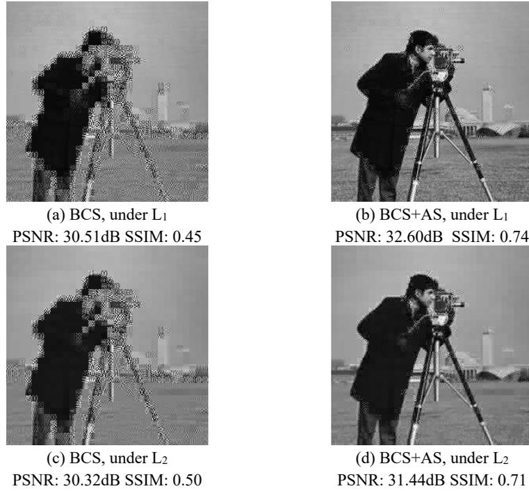
**Fig. 3.** Simulations for BCS under  $L_1$  and  $L_2$  constraints for test image cameraman.
