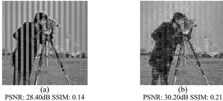
**Fig. 4.** Simulations of reconstructed image qualities for BCS with adaptive sampling under the  $L_1$  constraint for lossy rate of 50%. (a) No protection applied. (b) Protection with MDTC.
