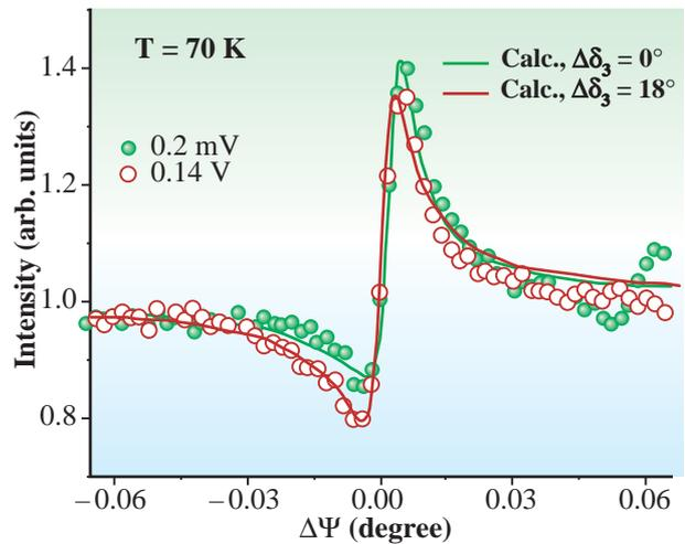
Fig. 2. Triplet phase change  $\Delta\delta_3$  extrapolated from curve fitting of the 3-wave diffraction profiles of the primary reflection  $\mathbf{G}_1 = (13\ q\ -6.5)$  at  $V = 0.2\ \text{mV}$  and  $0.14\ \text{V}$ . The analysis is based on the dynamical theory for multiple diffractions [7].
