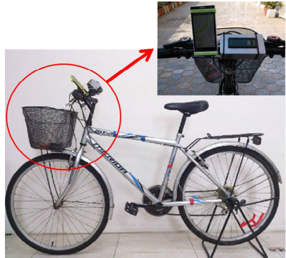
Fig. 7. Image of the bicycle-based event data recorder
