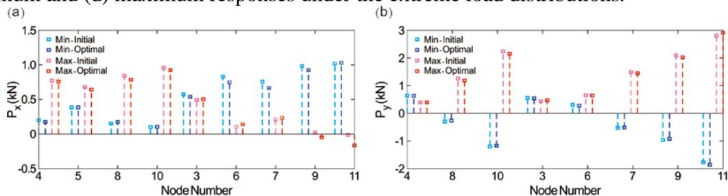
Figure 3: Load distributions to the peak responses of  $x_2$ -component deformation at node no.11 of the initial and optimal structural designs. (a) The extreme load distributions of  $x_1$ -component and (b) the extreme load distributions of  $x_2$ -component.
