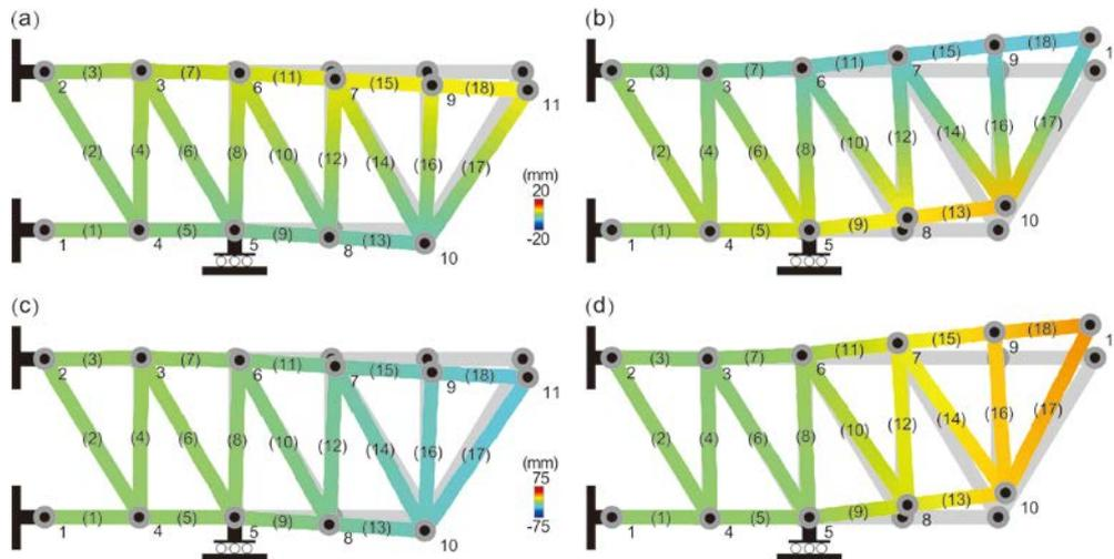
Figure 2: Structural peak response of  $x_2$ -component deformation at node no.11: Deformation fields of  $x_1$ -component corresponding to the structural (a) minimum and (b) maximum responses, and deformation fields of  $x_2$ -component corresponding to the structural (c) minimum and (d) maximum responses under the extreme load distributions.
