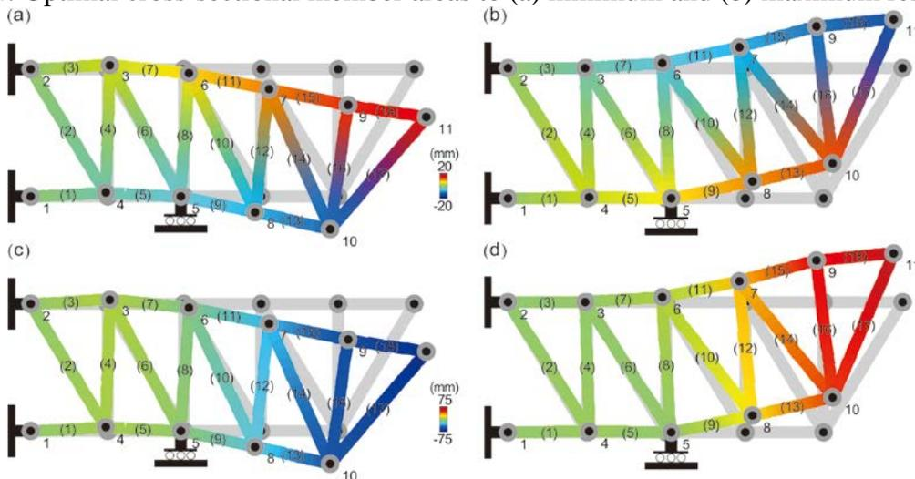
Figure 5: Structural peak response of  $x_2$ -component deformation at node no.11 of the optimal design: Deformation fields of  $x_1$ -component corresponding to the structural (a) minimum and (b) maximum responses, and deformation fields of  $x_2$ -component corresponding to the structural (c) minimum and (d) maximum responses under the extreme load distributions.
