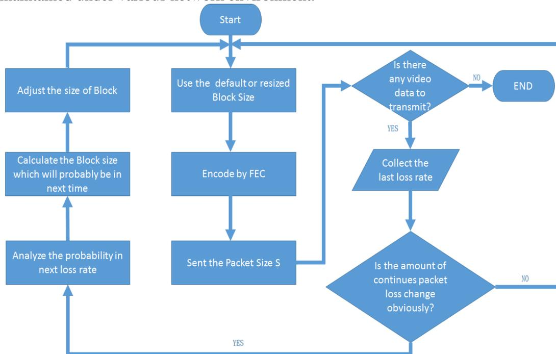
Figure 3. Dynamically adjust the block size flowchart
