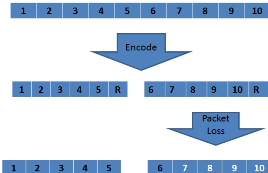
Figure 1. The original FEC mechanism
