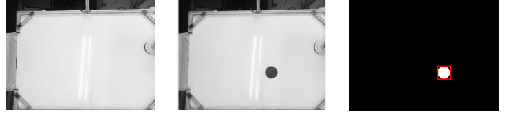
(a) Background Gray Image (b) Input Gray Image (c) Operation Output Fig. 2. Illustration of background subtraction algorithm.
